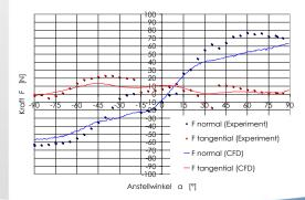
The primary target of the current study was to determine the forces and moments for real wind conditions and all possible positions of different barrier with respect to the ground. To maximize the accuracy all fluid dynamical effects like vortices at the inner structure and the barrier tips has been taken into account.
