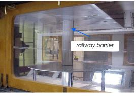
arm and the generated aerodynamic forces. For this a part of the barrier arm has been placed in the measurement section of the wind tunnel and connected to a weighing system, which is able to measure 3 forces and 3 moments simultaneously with an accuracy of 0,01 Newton. This system also allowed the barrier to be rotated around its longitudinal axis.
