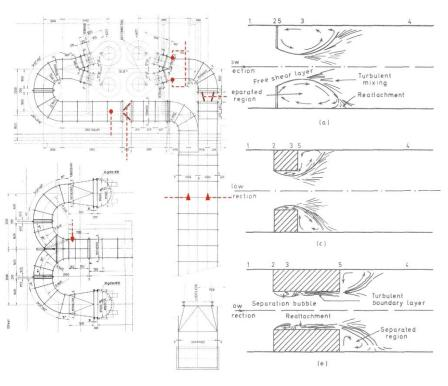
FlowMotion has therefore been asked to look for the reasons for this costly malfunction. To get a deeper insight in the fluid dynamical effects within the system velocity and static pressure measurements have been performed during the preliminary phase of the project. The measurement points have been set at fluid dynamical critical positions the channels.
