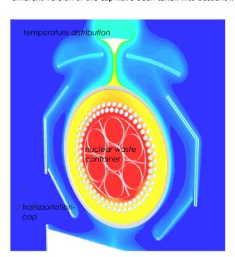
FlowMotion has simulated the air flow in and outside the cap and the resulting total heat dissipation of the container with the help of CFD (Computational Fluid Dynamics) calculations. In these simulations free convectional flow along all components no approximation by heat transfer coefficients), thermal conduction within the solids and thermal radiation have been calculated.
