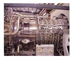
The design of the ventilation system of a GT enclosure is particularly complex, because many different requirements have to be fulfilled. In the first place the enclosure, which is barely larger than the turbine itself, protects the surroundings from the enormous heat and noise level emitted from the turbine. The amount of thermal energy can exceed 1 MW for certain gas turbines.
