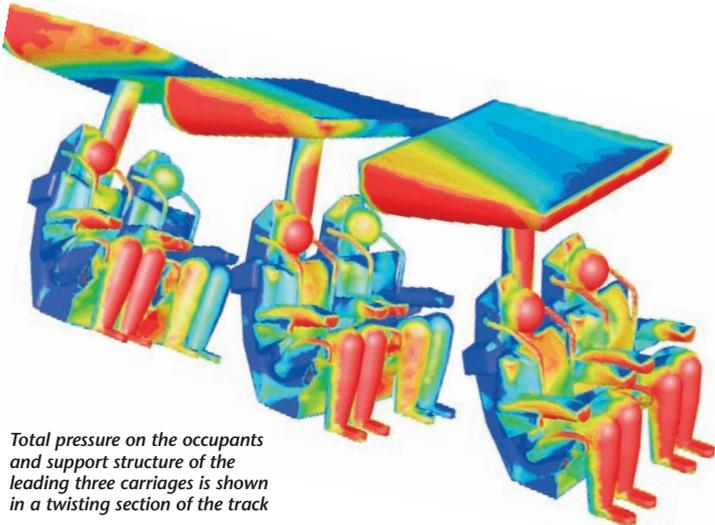
Total pressure on the occupants and support structure of the leading three carriages is shown in a twisting section of the track
